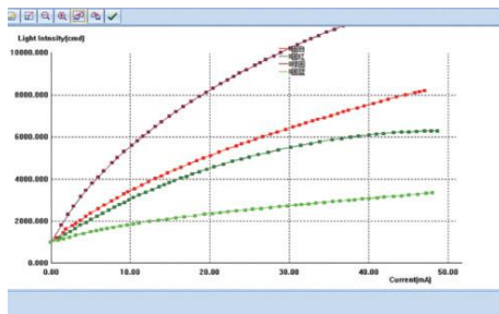
The curve showing the variation of the average light intensity in one-dimensional space with the current
